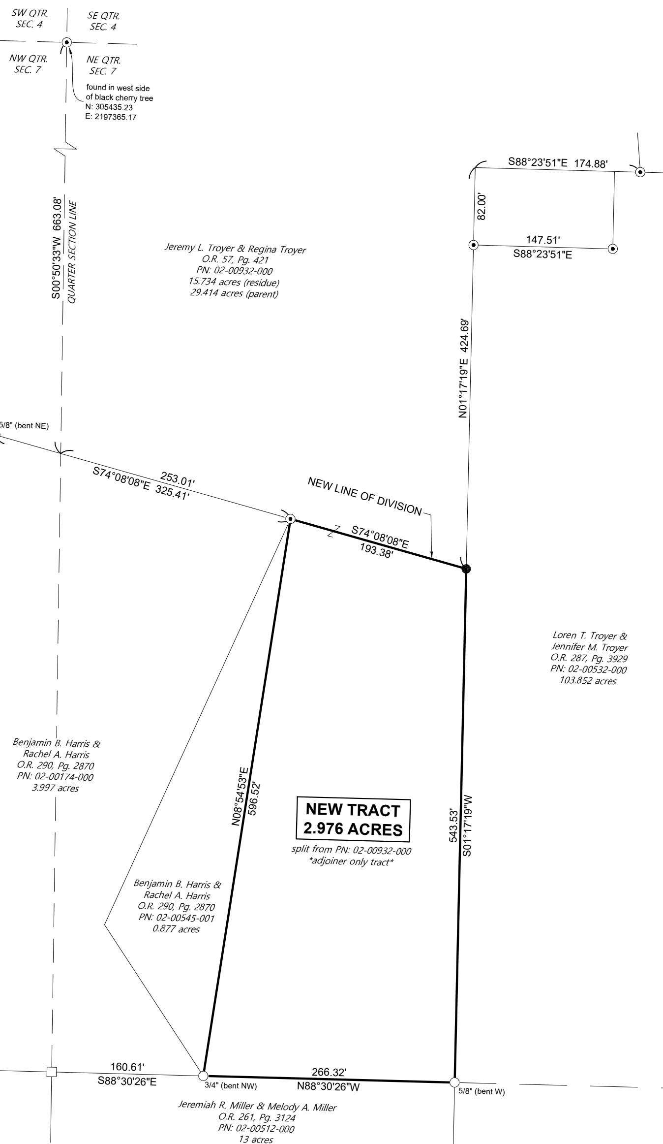
The Basis of Bearings is Grid North of the Ohio State Plane Coordinate System, NAD83(2011), North Zone as resolved through GNSS observations using the ODOT VRS Network.
